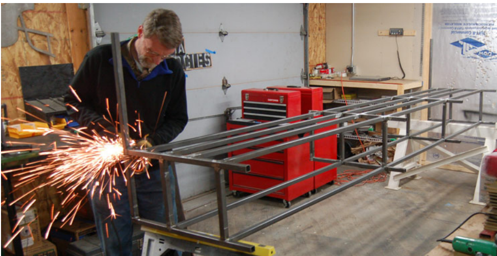
Dave, WA1ZCN, grinding welds on the trailer bench frame
