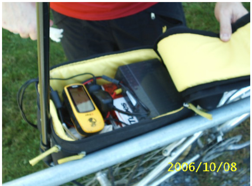
Part of the APRS setup used by KX1Y Garmin eTrex, AGM battery and bike antenna Front bike bag held TH-D7A and hand mic (not pictured)
